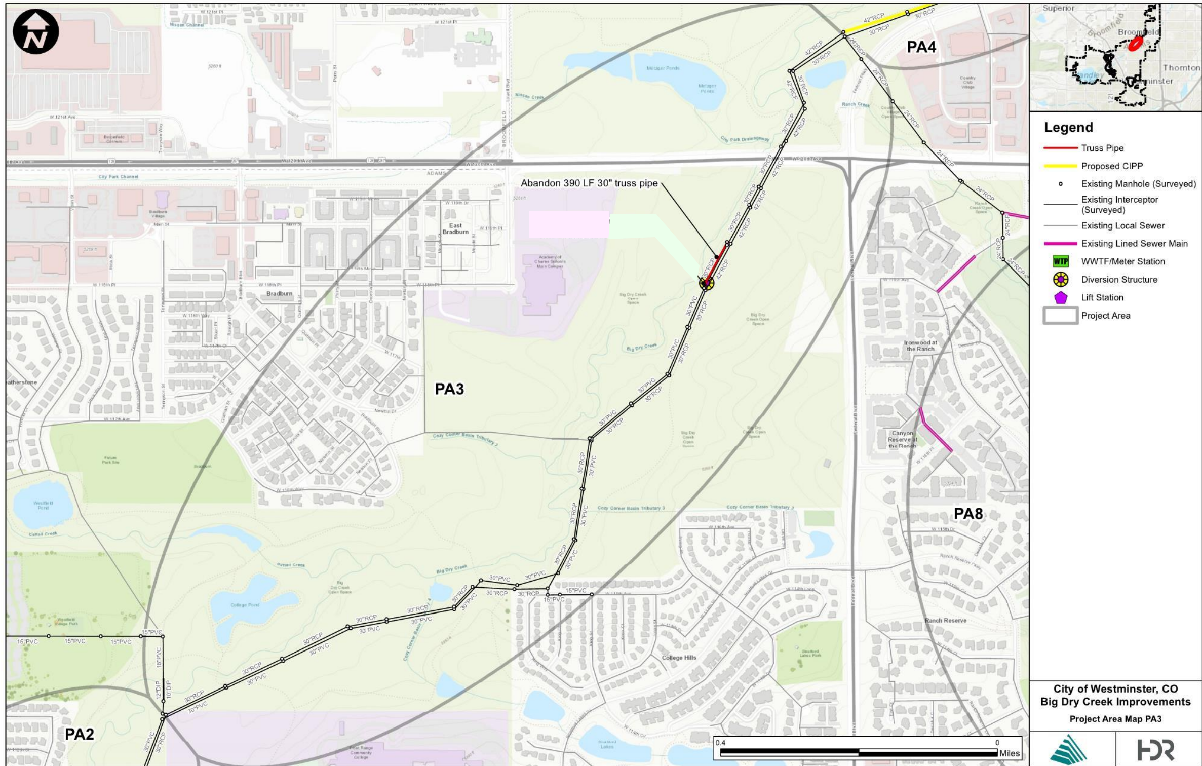
Figure 5. Project Area 3 – Recommended Alternative – Abandon 300-FT of Truss Pipe
